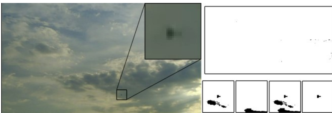
Figure 3.15 Example of the situation with high contrast clouds: on the left the original image with the enlarged aircraft, on the upper right the result of first adaptive threshold, on bottom right from left to the right the darker pixels, brighter pixels, OR operation and the segmented aircraft
