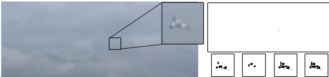
Figure 3.14 Example of the situation with medium contrast clouds: on the left the original image with the enlarged aircraft; on the upper right the result of first adaptive threshold, on bottom right from left to the right the darker pixels, brighter pixels, OR operation and the segmented aircraft
