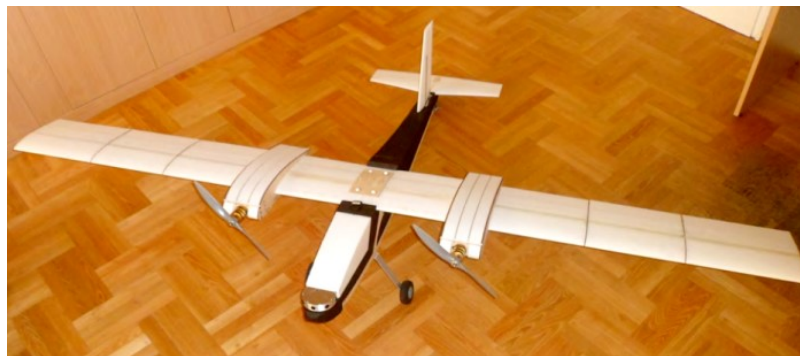
Figure 7.1 The aircraft called Orca, the five camera system can be seen on the nose of the fuselage
